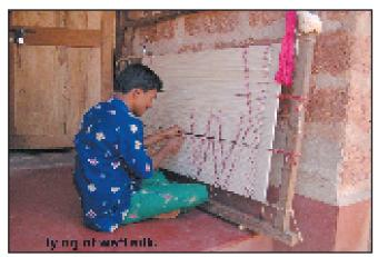
in kera form in the wooden frame and tied with twisted yarn the portions, which need to be left white in the design. This process is repeated depending upon the number of colours required in the design. Then dying of yarn is carried out. Mostly Direct, Acid and Metal complex dyestuffs are used in the cluster during tie and dye process. However Metal complex dyes are now widely used for its good fastness properties and wide range of sales. All
