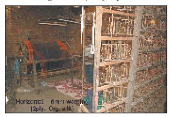
obtained are passed through sizing process (using, fried rice) and wound to a stick cage, which takes further 8-10days. The yarn on the stick cage is dried. This stick cage process is too laborious, it adds a lot to the cost price of the product. Automatic winders can be introduced to do this job, first in experimental basis and then in commercial basis till subgrouping of ikat process.
